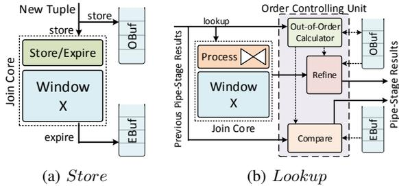
Fig. 5: Order control unit architecture.
